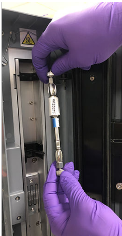
Figure 8–60: Installing the replacement column
