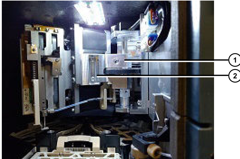
Figure 8–44: Magnet location in needle carriage arm
